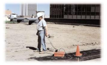
The instrument consists of a transportable field electromagnetic impulse transmitter and receiver, which emits impulses that are reflected back to the receiver. The returned impulse-variations are presented as hyperbolic patterns, caused by the reflection changes, and are displayed graphically on a strip chart. This provides paper documentation and gives a continuous record of the subsurface under the track of the antenna.
